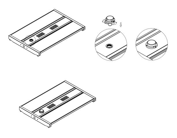
b. Twist the sensor clockwise into the socket .
