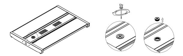
a. Remove the sensor cover (use a Phillips screw driver and turn counter clockwise to remove).
