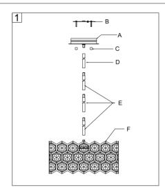
2. Connect mounting bracket (B) to the outlet box with short machine screws (BB).
