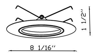
**LAMPING:** Accommodates a PAR38 E26 100 W Max. Please see housing for maximum wattage allowed according to selection.
